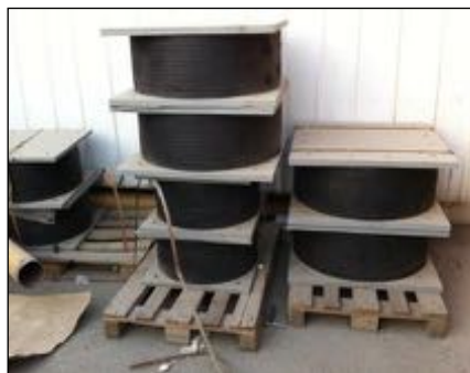
Figure 1. Lead-rubber bearings with different dimension
